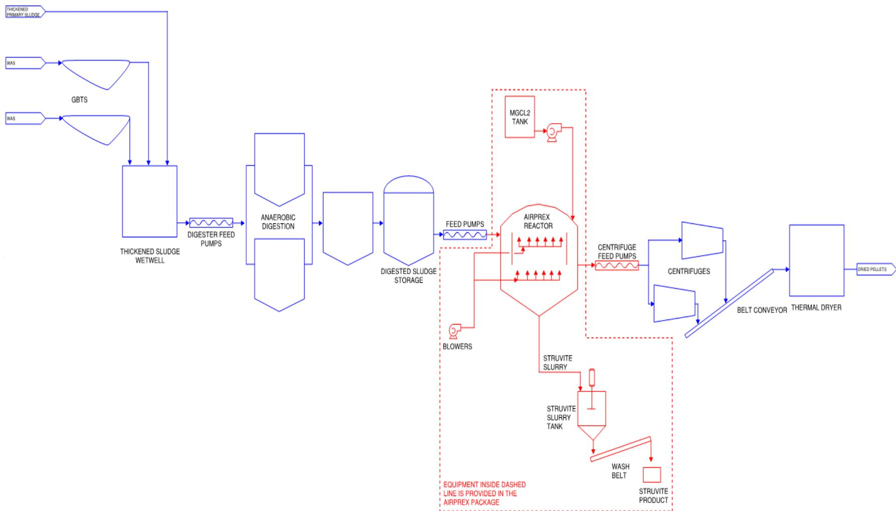
Figure 1-12: Blue Lake WWTP proposed flow diagram for phosphorus management approaches using biosolids harvesting/sequestration technologies.
