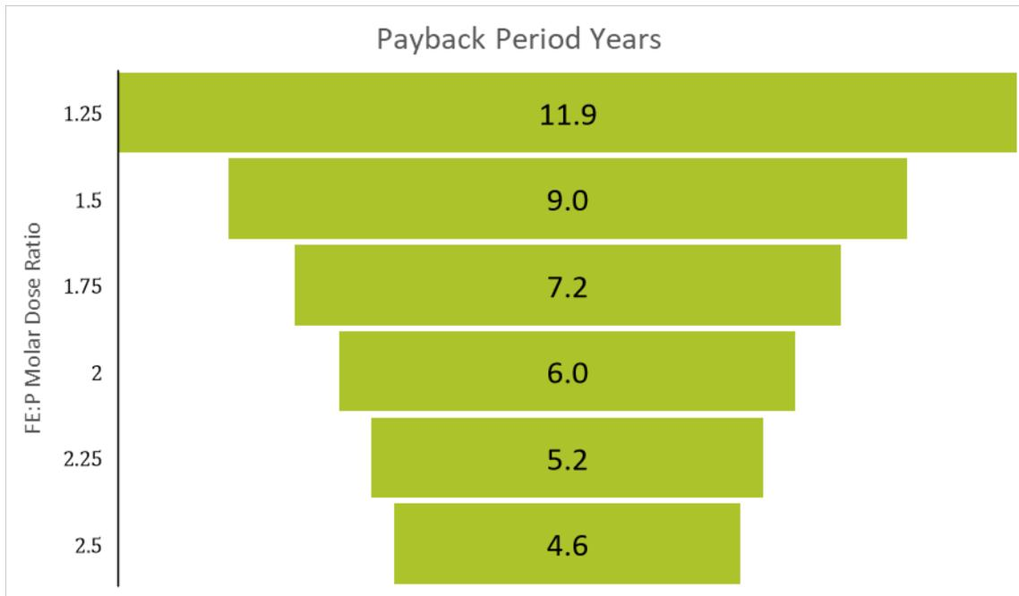
Figure 1-20: Struvite harvesting alternative payback period impact related to comparison of the status quo and ferric dosing ratio. Payback period used for cost comparisons was 6 years, a molar ratio of 2.0.
