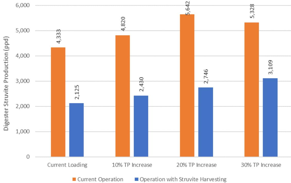
Figure 1-16: Comparison of struvite harvesting/sequestration technologies vs. current operation of digester struvite production with increasing phosphorus loading.
