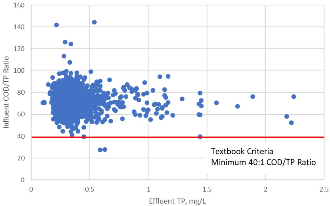
Figure 1-4: Blue Lake WWTP historical influent BOD/TP ratio vs. effluent total phosphorus. Data available from January 2014 through September 2018.
