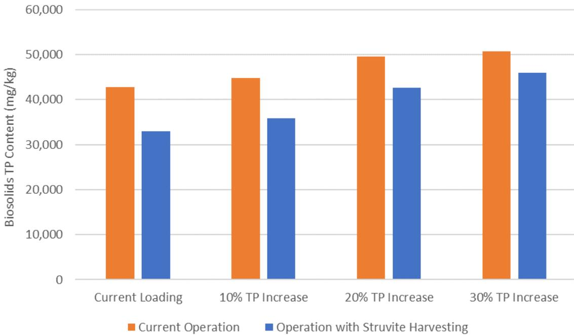
Figure 1-18: Final biosolids phosphorus content of current operation vs. struvite harvesting technologies for the eight evaluation scenarios.
