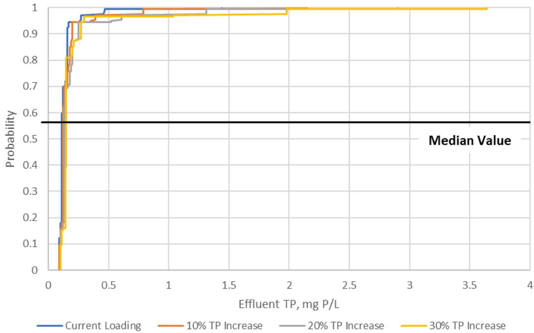
Figure 1-13: PT simulation results of Scenarios 5-8 with struvite harvesting/sequestration technologies.
