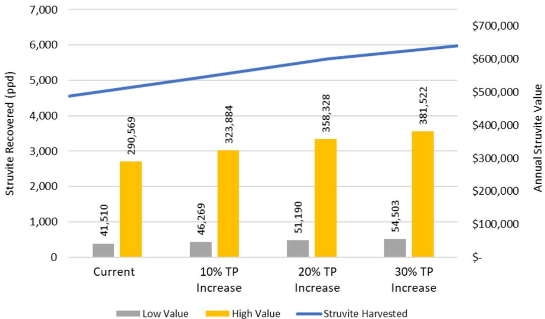
Figure 1-17: Potential value of struvite harvesting technologies based on the percent of struvite recovered. Percent recoveries assumed a range including 30%, 40%, and 50%.
