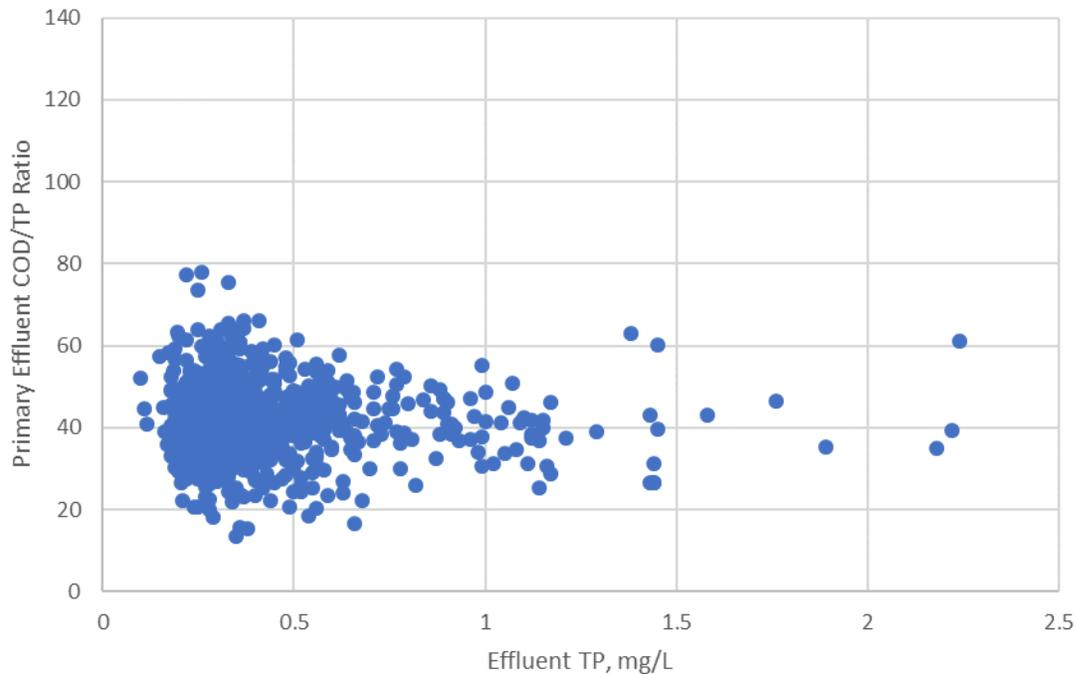
Figure 1-7: Blue Lake WWTP primary effluent COD to influent TP ratio vs. effluent total phosphorus. Data available from January 2014 through September 2018.
