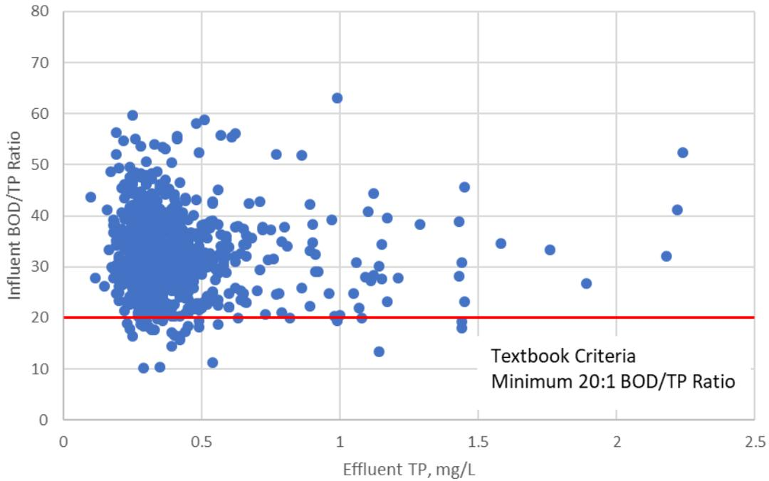
Figure 1-3: Blue Lake WWTP historical influent BOD/TP ratio vs. effluent total phosphorus. Data available from January 2014 through September 2018.
