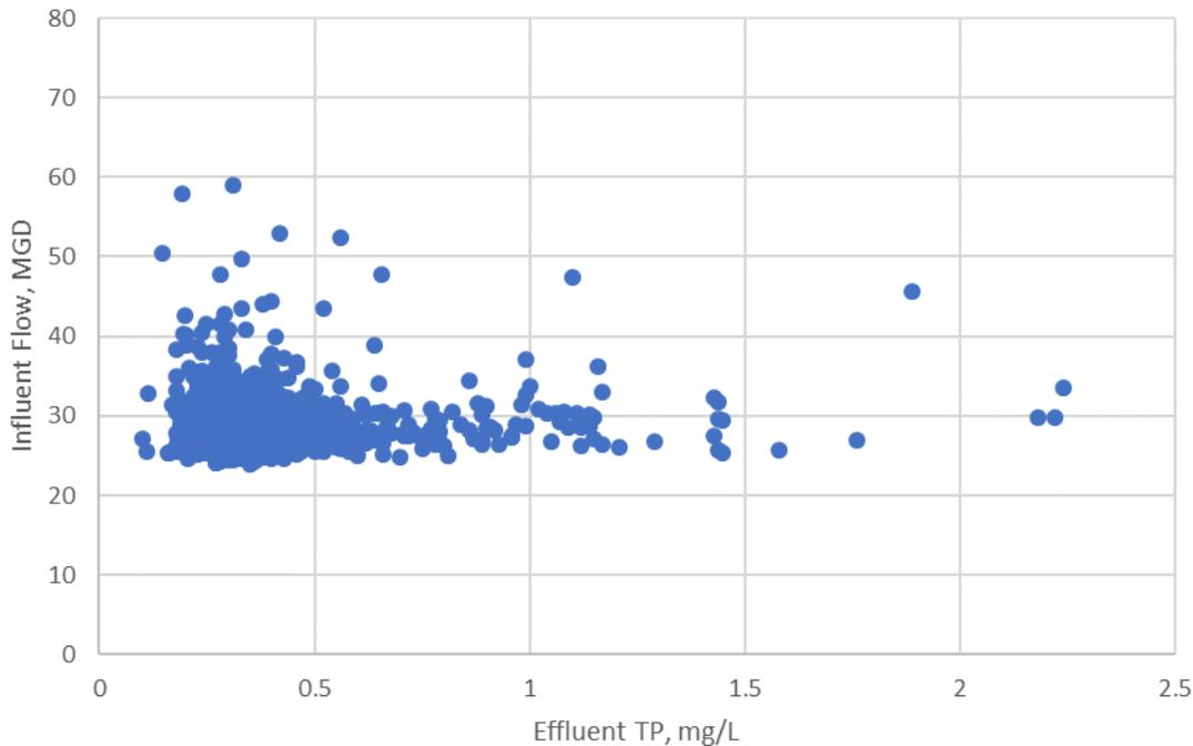
Figure 1-8: Blue Lake WWTP influent flow vs. effluent total phosphorus concentration. Data available from January 2014 through September 2018.
