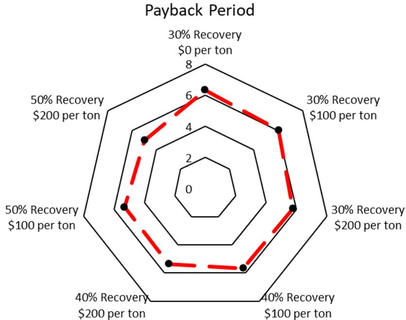
Figure 1-21: Struvite harvesting alternative payback period variability related to product recovery and value. Payback period used for cost comparisons assumed 30% recovery at a value of \$100 per ton.
