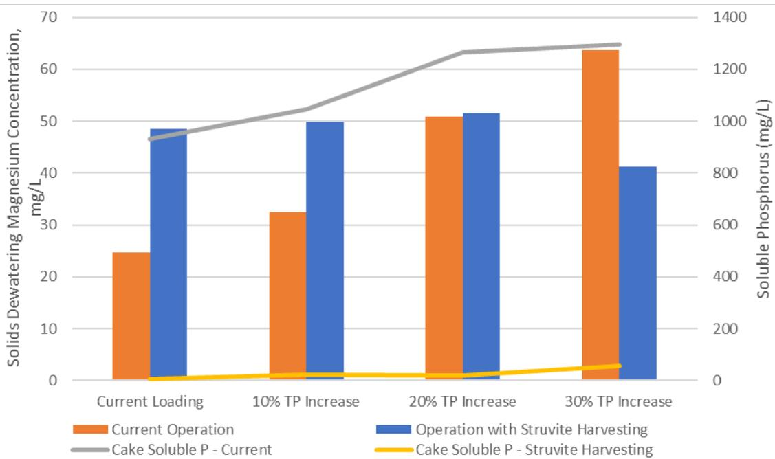
Figure 1-19: Final biosolids phosphorus and magnesium concentrations for both current operation and implementation of a struvite harvesting/sequestration technology.
