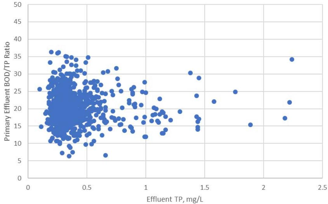
Figure 1-6: Blue Lake WWTP primary effluent BOD to influent TP ratio vs. effluent total phosphorus. Data available from January 2014 through September 2018.
