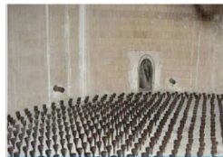
Fluid Bed Incinerator Rehabilitation
