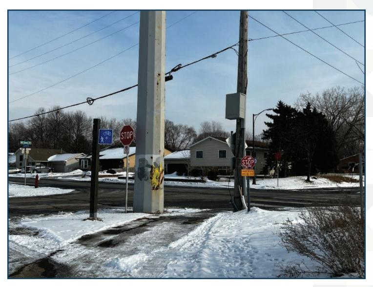
East Bank Trail existing intersection with Plymouth Avenue obscured by transmission towers. Intersection design will mitigate sightline issues through curbline shifts, reduce crossing distance from 52 to 26 feet and incorporate overhead crossing signage and RRFBs to enhance crosswalk visibility and safety of trail users.
