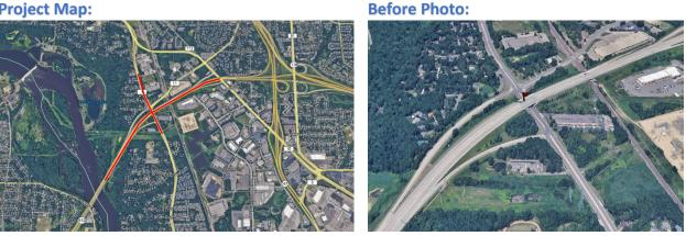
Project Description: The project will complete the transportation system by providing a full-access interchange at TH 610 and East River Road with a westbound off-ramp loop and a folded eastbound onramp with TH 610 auxiliary lanes between East River Road and Coon Rapids Boulevard. In addition, multimodal improvements include the construction of a new 10-foot trail along the East River Road corridor.
