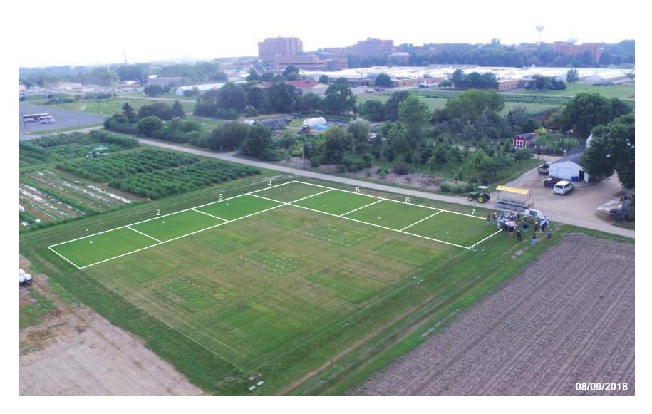
Figure 1. The project location at the turfgrass research farm on the UMN St. Paul campus. The irrigation treatments were a regular time-based Controller A (1), Smart Controller B (2), Smart Controller C + Rain Sensor (3), a non-irrigated plot (4), Smart Controller D (5), a manually-irrigated plot (6), and Soil Moisture Sensor + Controller F (7).
