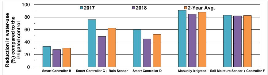
Figure 5. Reduction (%) of various irrigation technologies and manual irrigation relative to the irrigated control during 2017 and 2018. 2017 trial ran from July 15 to October 19 (97 days). It is likely some irrigation ran that was unaccounted for and was not part of the scheduled program (such as following fertilizer applications or for demonstration purposes). 2018 trial ran from June 4 to October 5 (124 days).
