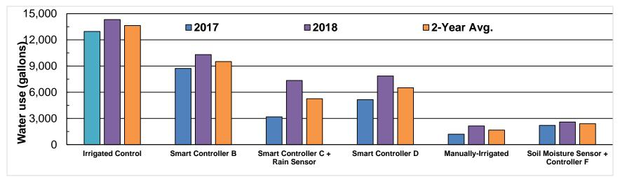
Figure 4. Water use (gallons) of various irrigation technologies and manual irrigation compared to irrigated control during 2017 and 2018. 2017 trial ran from July 15 to October 19 (97 days). It is likely some irrigation ran that was unaccounted for and was not part of the scheduled program (such as following fertilizer applications or for demonstration purposes). 2018 trial ran from June 4 to October 5 (124 days).
