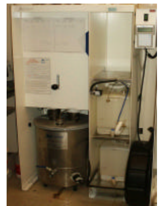
Solvent recycling units installed and in operation at Abbott Northwestern Hospital Laboratory.
