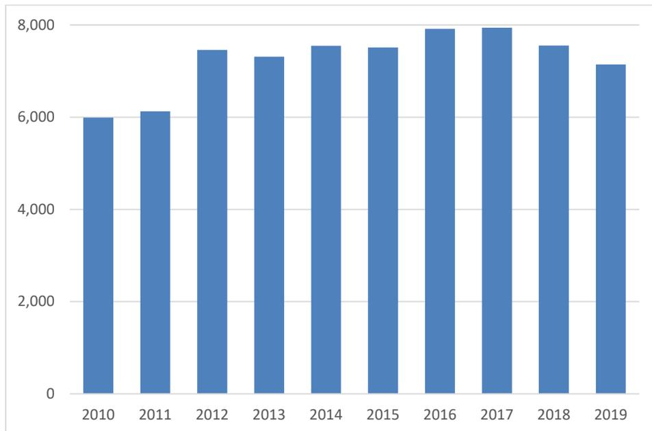
Note: Mileage is the distance traveled in service between mechanical failures. Higher is better.
