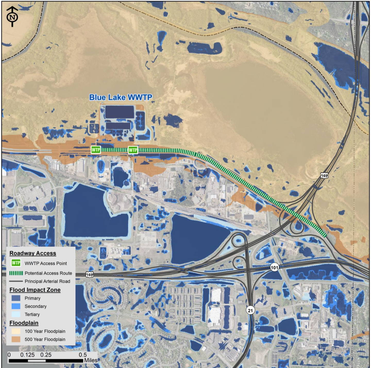
Figure 3. Blue Lake Wastewater Treatment Plant Potential Localized Flooding
