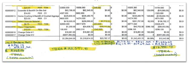
The example above illustrates how an AIA continuation sheet should be annotated. Notice that the retainage amounts are clearly indicated so the net amounts claimed are understandable and that the line items claimed are highlighted.
