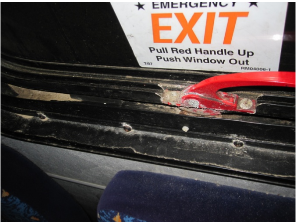
Fig 3.1 Corroded Emergency exit handles
