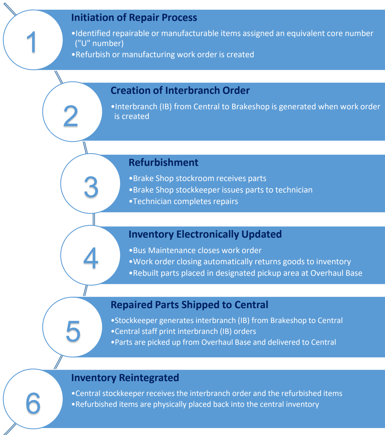
Figure Eight: Manufactured Parts Process Flow 11
