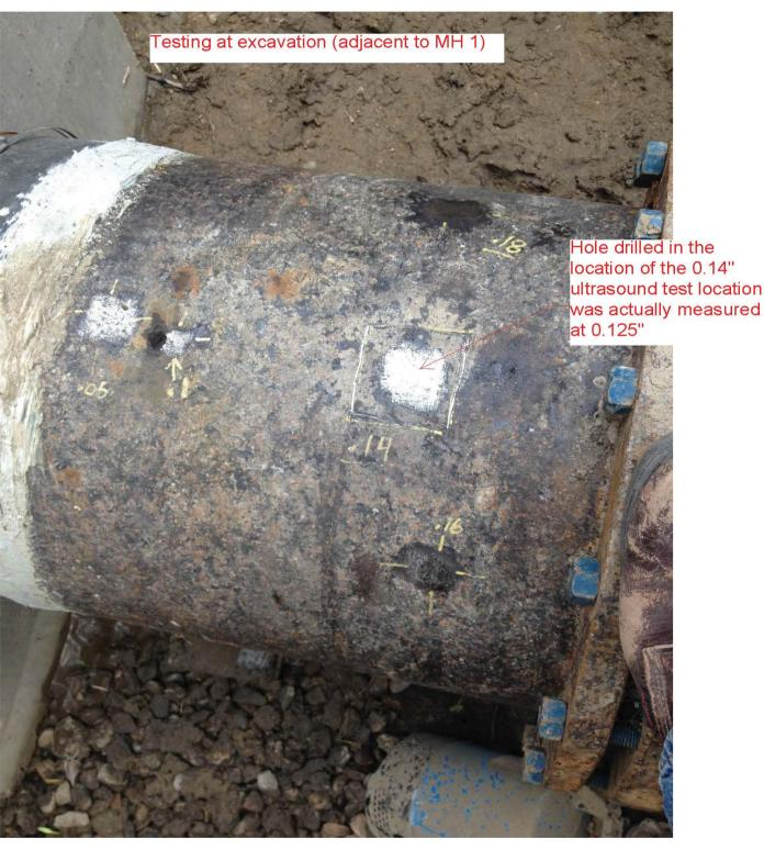
Additionally, the 20" DIP, CL.52 spool piece pipe at Magney's trailer was measured to verify accuracy of ultrasound. It measured 0.44" and 0.45" where factory is 0.42". Also, the coupon from Phase 2 (SJ Louis) conveyance which was on the DIP portion measured 0.51" in thickness while the ultrasound gave readings ranging from 0.52" to 0.54".
