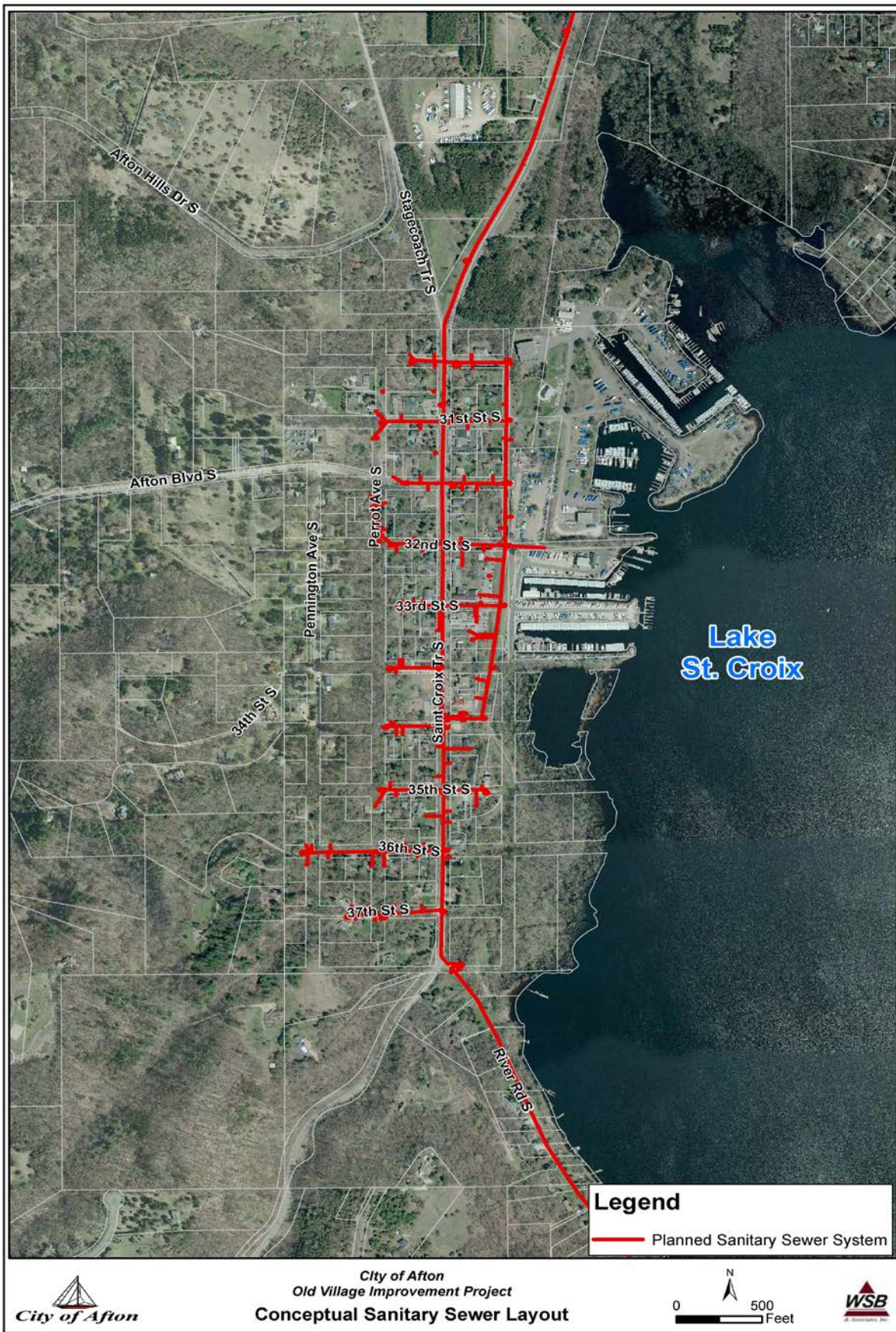
Figure 4: Conceptual Sanitary Sewer Layout
