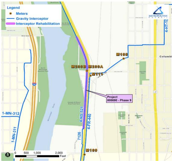
Line 4,300 lineal feet of 96-inch diameter concrete pipe by cured in place pipe method
