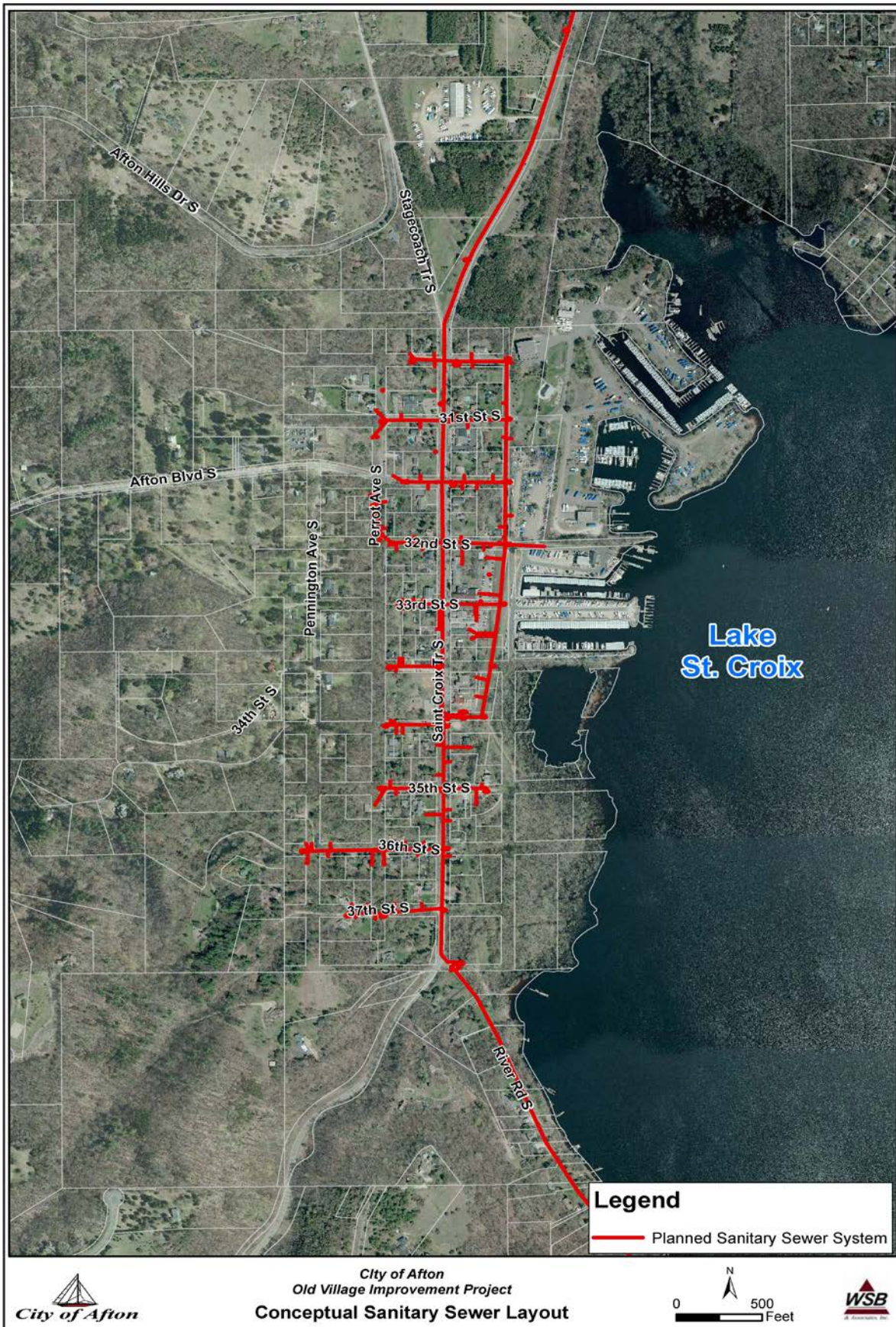
Figure 4: Conceptual Sanitary Sewer Layout
