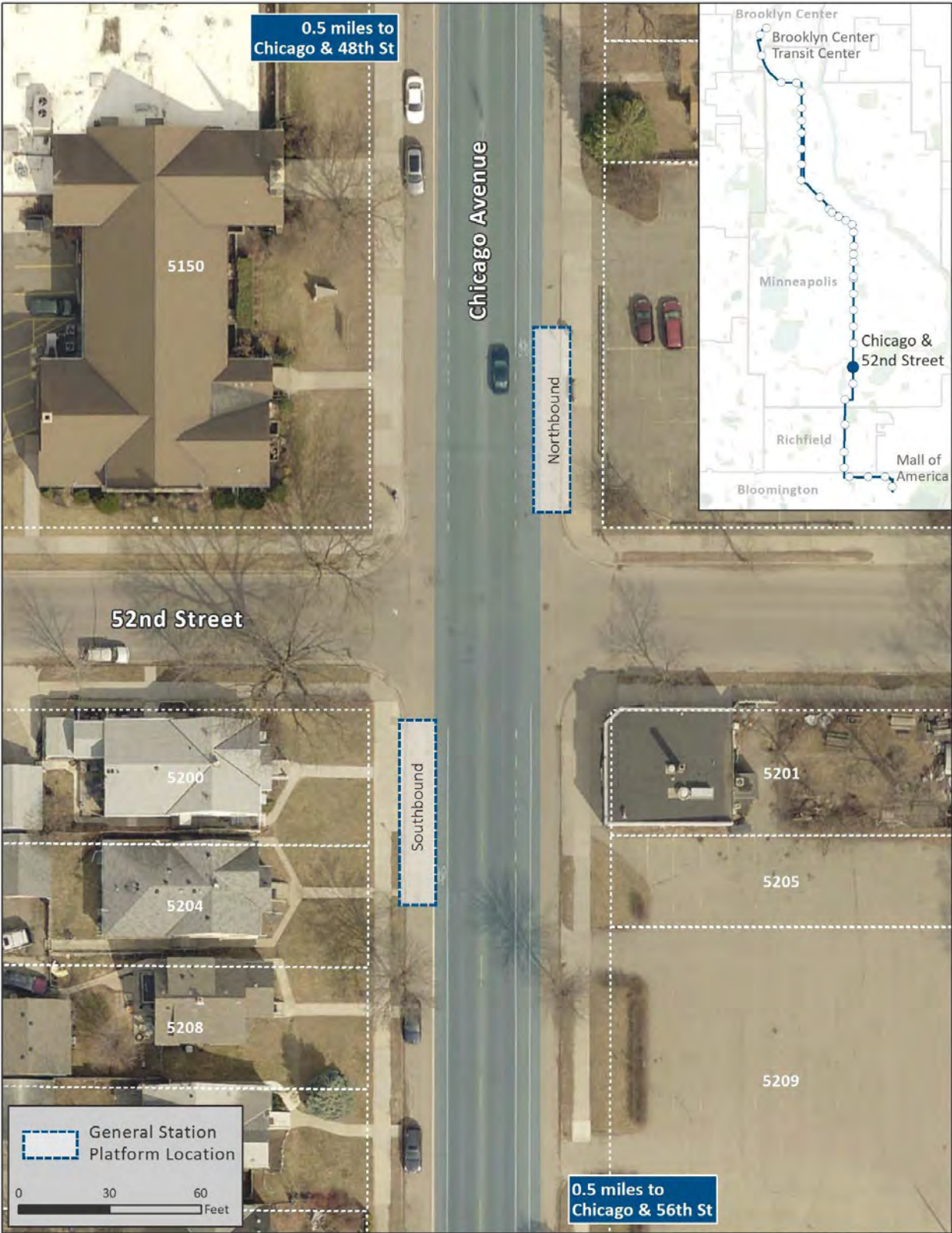
Figure 49: Recommended station location - Chicago & 52nd Street
