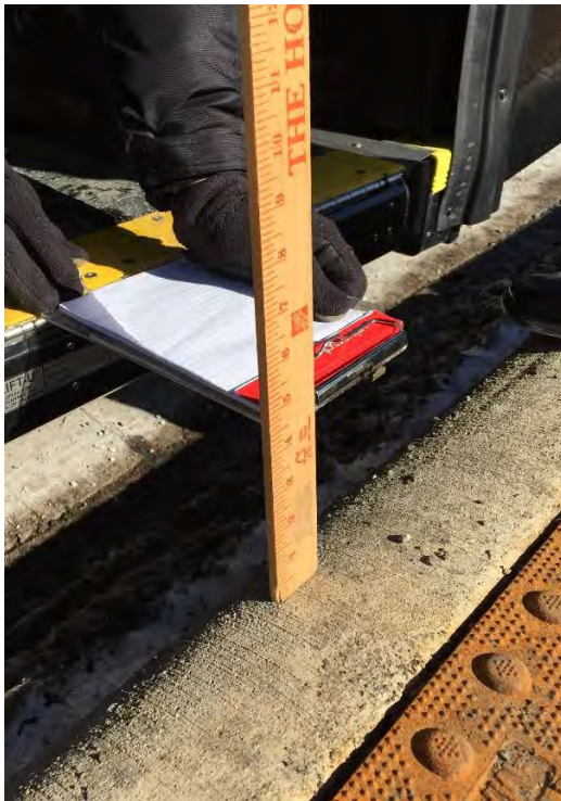
Figure 15: Near-level boarding detail
