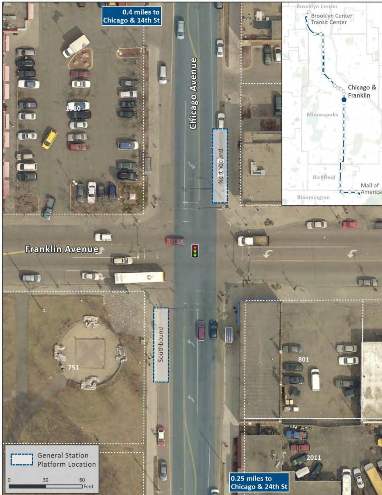
Figure 38: Recommended station location - Chicago & Franklin
