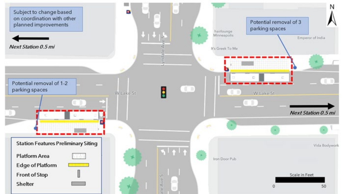
Nearside platform location example (recommended corridor plan)
