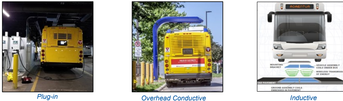
Figure 12: BEB charging infrastructure
