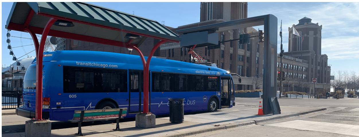
Figure 22: Chicago Transit Authority Proterra BEB with overhead charger
