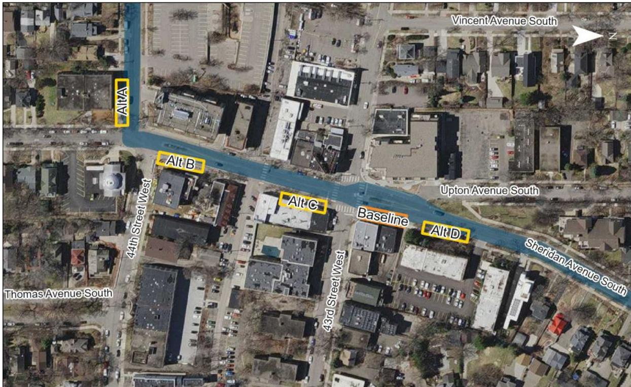
Northbound Alternatives A and B were not carried forward because platform construction is not feasible at these locations. The existing sidewalk and boulevard are too narrow to accommodate a platform within the existing curb line and expanding the platform with a bumpout is not feasible due to intersection constraints.
