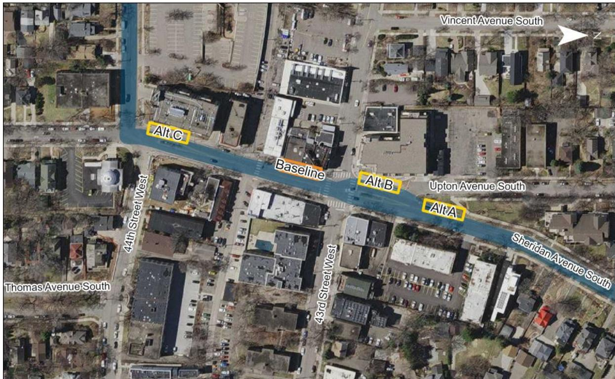
Southbound Alternative C was not carried forward because platform construction is not feasible at this location. The existing sidewalk and boulevard are too narrow to accommodate a platform within the existing curb line and expanding the sidewalk with a bumpout is not feasible due to intersection constraints. Additionally, there is a steep uphill grade at this platform location.
