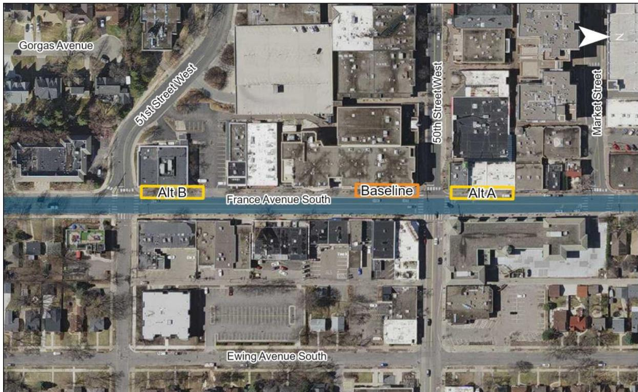
Southbound Alternative A on France Avenue and 50th Street nearside was not carried forward because platform construction is not feasible without reducing the intersection to a single southbound lane and eliminating the left-turn lane onto eastbound 50th Street. The remaining alternatives were compared with the baseline platform location on the additional factors shown in Table 7.
