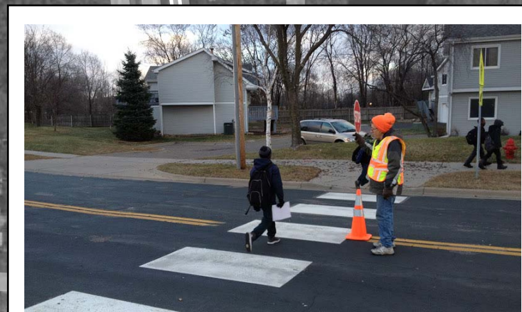
The location of this marked crossing on 70th Ave does not facilitate the current crossing behaviors of most students. Consider moving crosswalk to match existing crossing patterns or institute an education/enforcement program to shift behavior.
