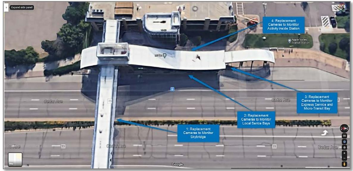
Figure 1 AVTS Camera Deployment Map, Northbound and Skybridge
