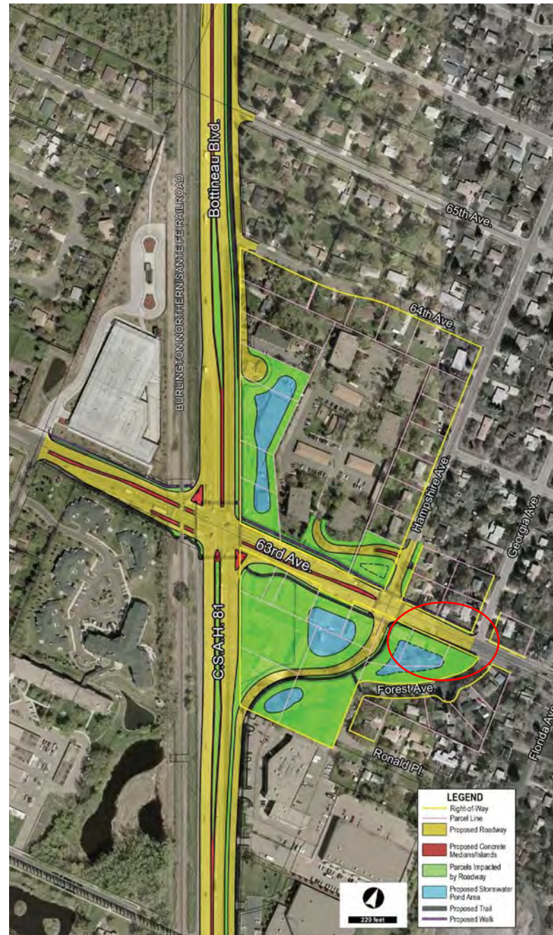
Figure 2 Bottineau Boulevard Reconstruction - Proposed Roadway Layout
