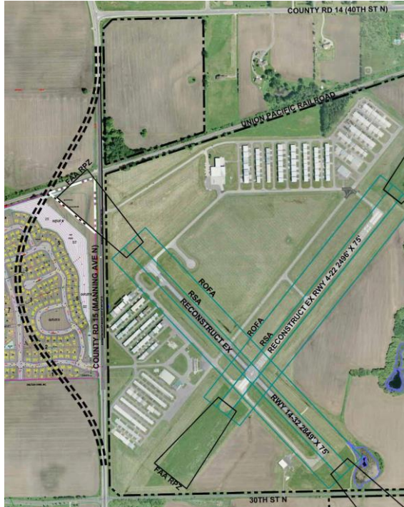
CONCEPTUAL MANNING AVENUE REALIGNMENT CORRIDOR TO CLEAR EXISTING RUNWAY PROTECTION ZONE (RPZ)
