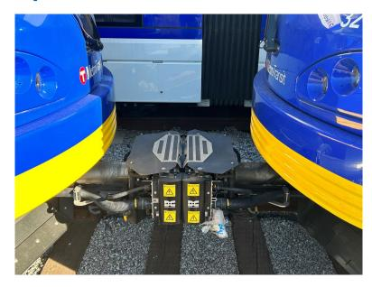
The automatic coupler joins vehicles together mechanically and electrically. The mechanical coupling is what physically connects the LRV's, while two electrical couplers transmit electrical signals between the coupled vehicles through cables. Coupling and uncoupling is carried out completely automatically.
