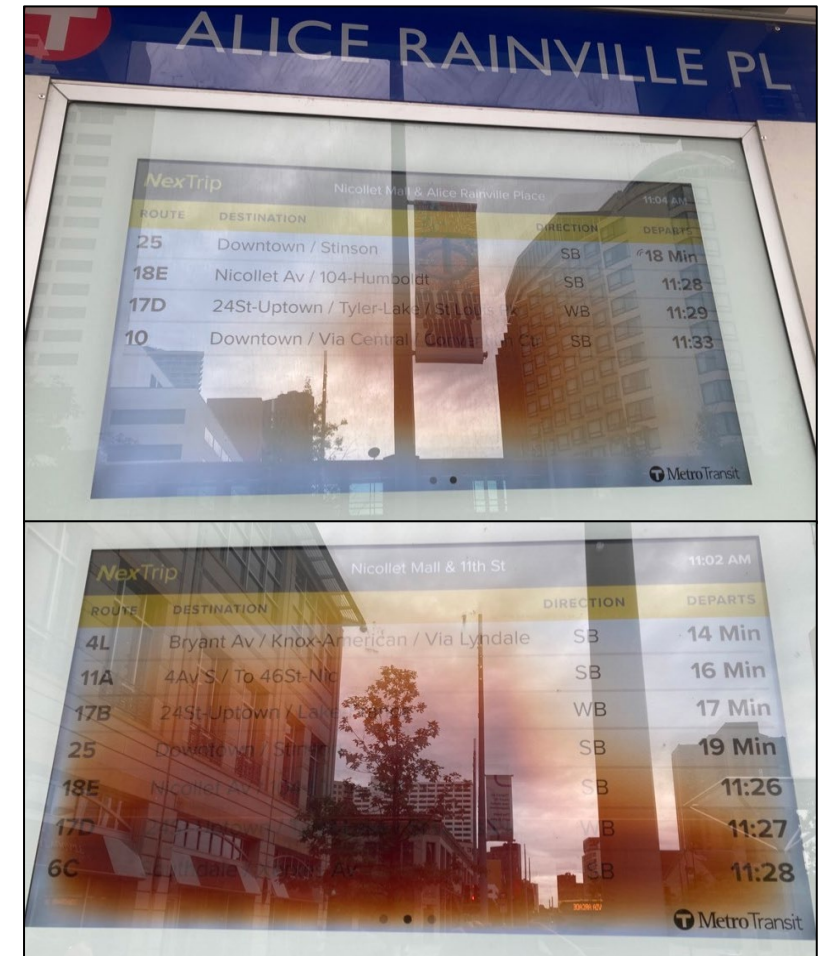
Image: Degraded screens along Nicollet Mall
