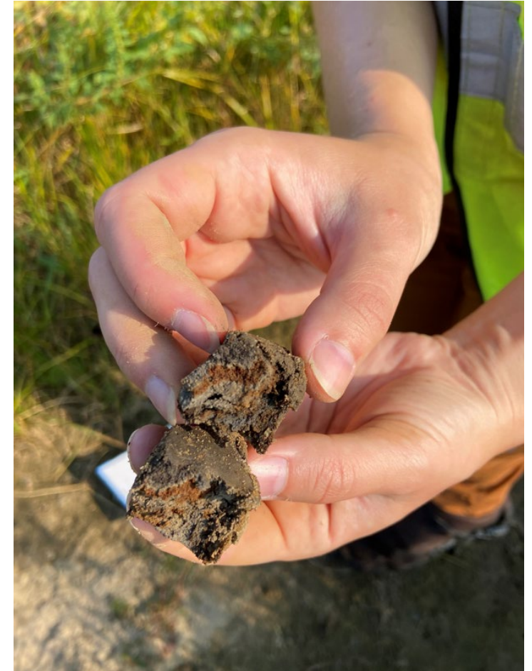
Example of soil boring used to identify soil types
