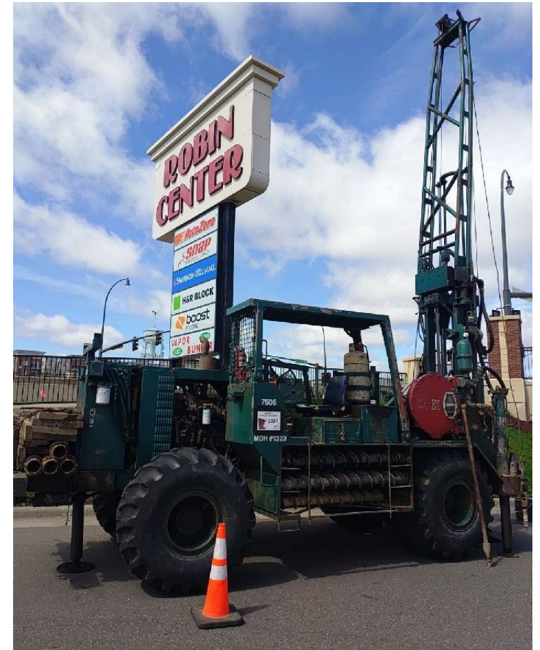
Image depicts equipment used for testing for contaminated soils
