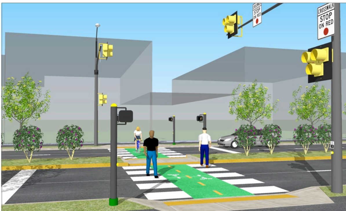
The Pedestrian Hybrid Beacon, or HAWK (in combination with crosswalk/crossbike treatments) would help people walking or on bicycles to cross major corridors such as Excelsior Boulevard.
