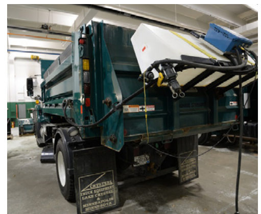
The cost saving from the City's creatively adapted brine sprayer was reinvested to purchase a more efficient and integrated fleet vehicle salt brine sprayer.
