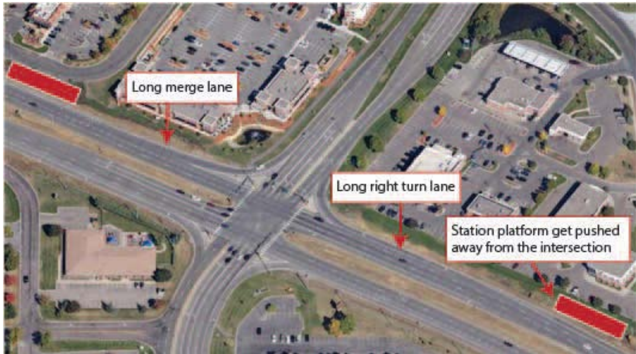
Figure 13: Typical Highway 55 Intersection Design
