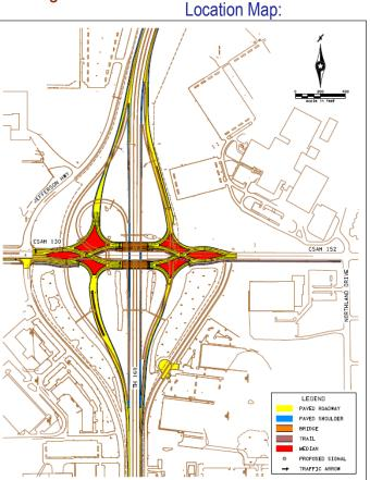
The proposed interchange improvements include the reconstruction and widening of the bridge over TH 169 to provide a diverging diamond interchange (DDI) with geometrically realigned ramps. There will be four westbound lanes and three eastbound lanes with the multi-use trail on the CSAH 130 bridge. Existing traffic signals will also be replaced at the TH 169 east and west ramp intersections. The DDI configuration will improve the overall capacity and safety of the interchange.
