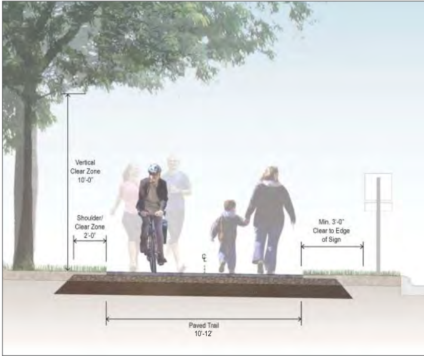
The West Edina Trail segment will be constructed as a 10-foot wide paved multi-use trail.
