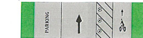
*2' GUTTER PAN / BITUMINOUS SEAMS (A1) EMERSON AVE N - PLYMOUTH AVE N TO 33RD AVE N (NEAR TERM BIKE LANE) -DESIGN EXCEPTION REQUIRED
