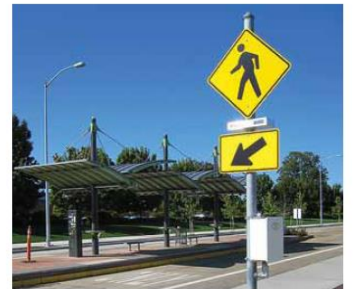
Rectangular Rapid Flash Beacons are a user activated flashing light, mounted to standard school crossing signs at crosswalks.
