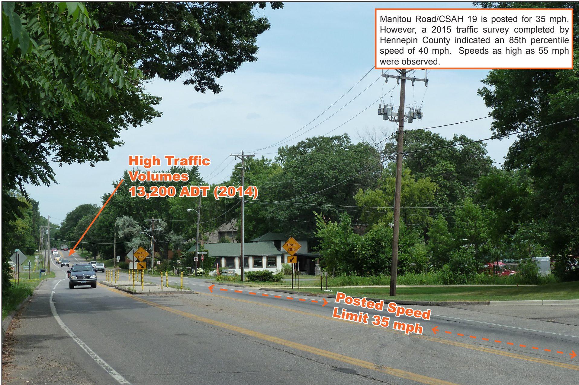
Site Photo - Manitou Road Approaching Lake Minnetonka LRT Regional Trail (Facing North)
