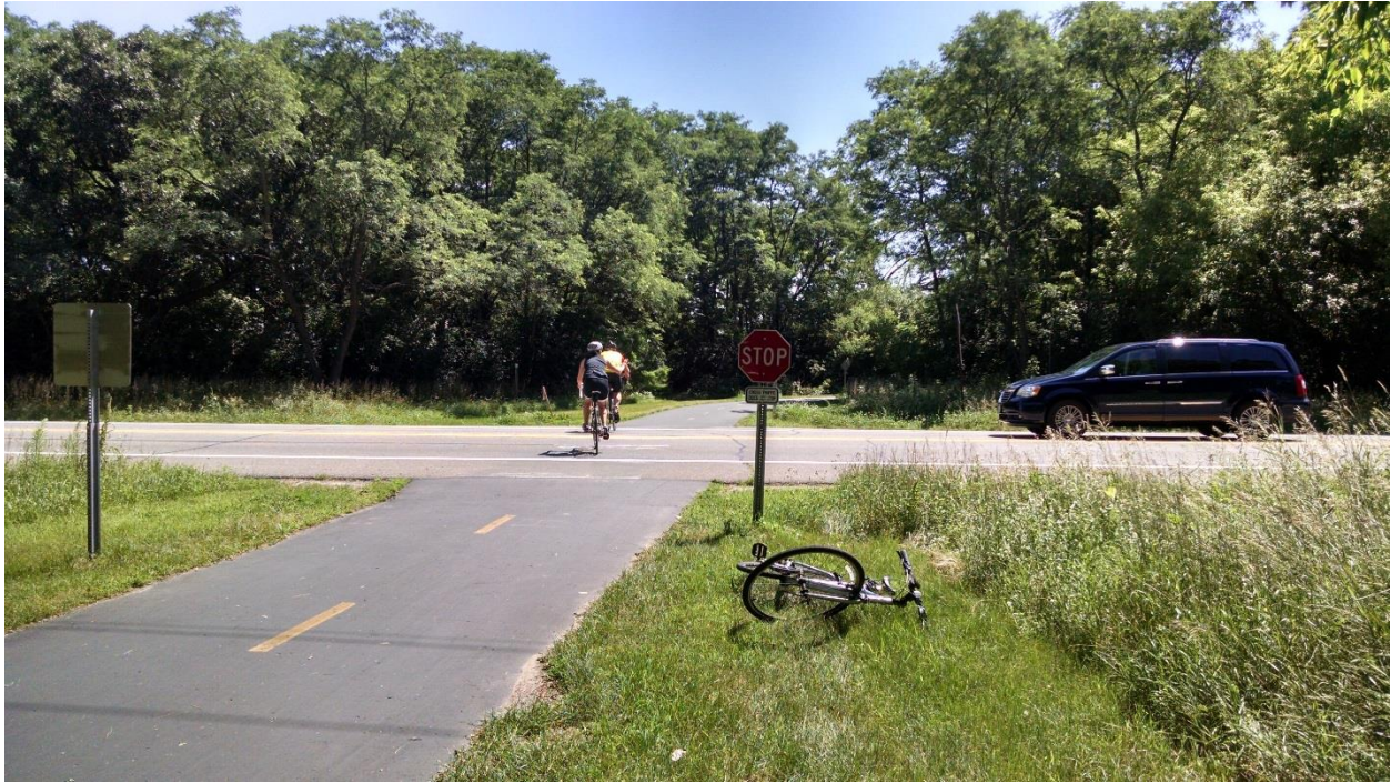
Rush Creek Trail – Winnetka Avenue North Crossing – View from the west looking east. Northbound traffic stopped on the 50 mph roadway creates an unsafe environment for trail users.
