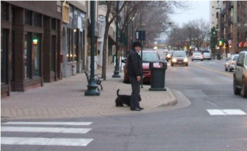
Curb extension, Hopkins, MN
