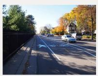
Typical existing cross section with the pedestrian space and bikeway separated from motor vehicle traffic by striping and plastic bollards.
