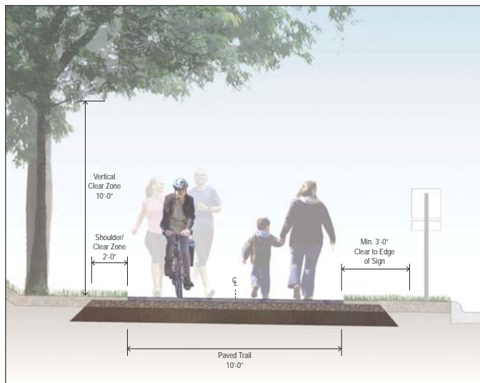
Figure 11: Typical Trail Cross-Section
