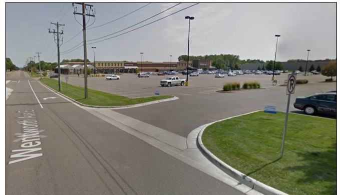
Sidewalk would be installed on the south side of Wentworth to provide connectivity for 0.5 miles through commercial, residential, and employment areas
