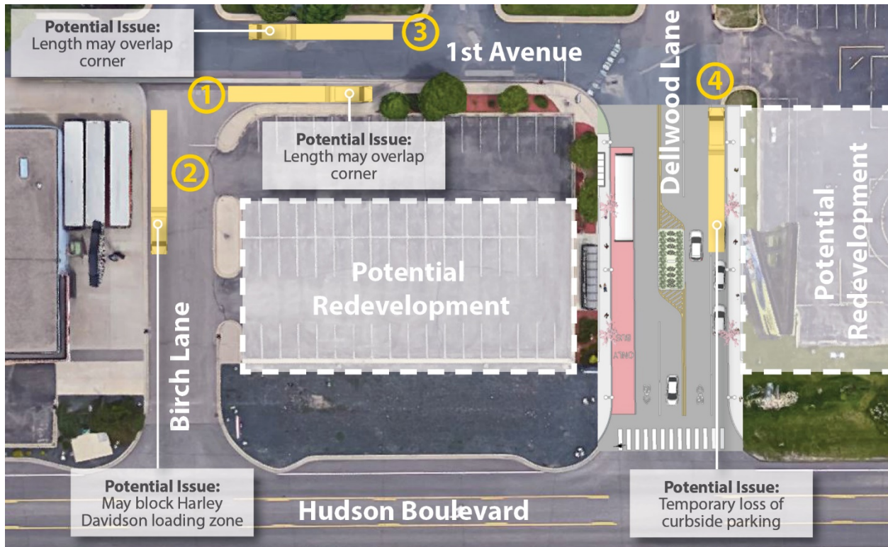
Figure 47. Options for Temporary Semi-Truck Parking
