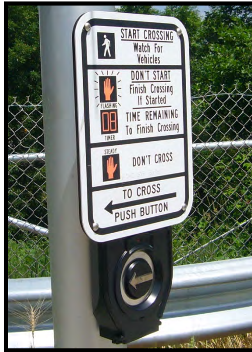
Figure C-5 Traffic Signal Pedestrian Phase
