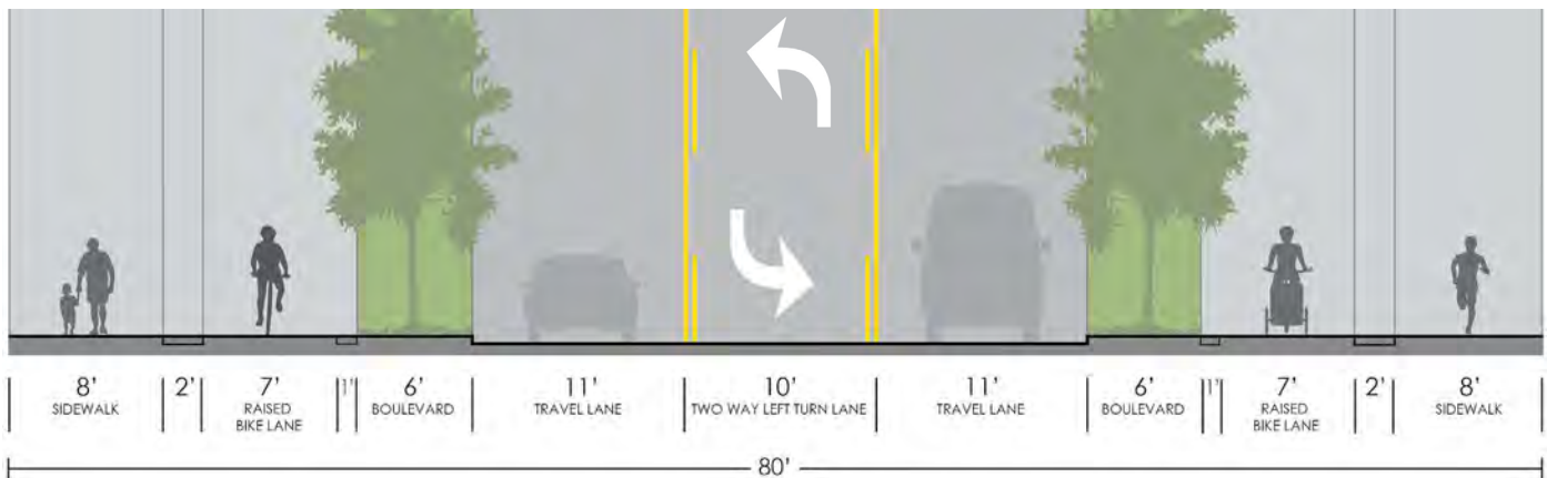
Figure 3.19 Section E: Vernon Avenue without median.
