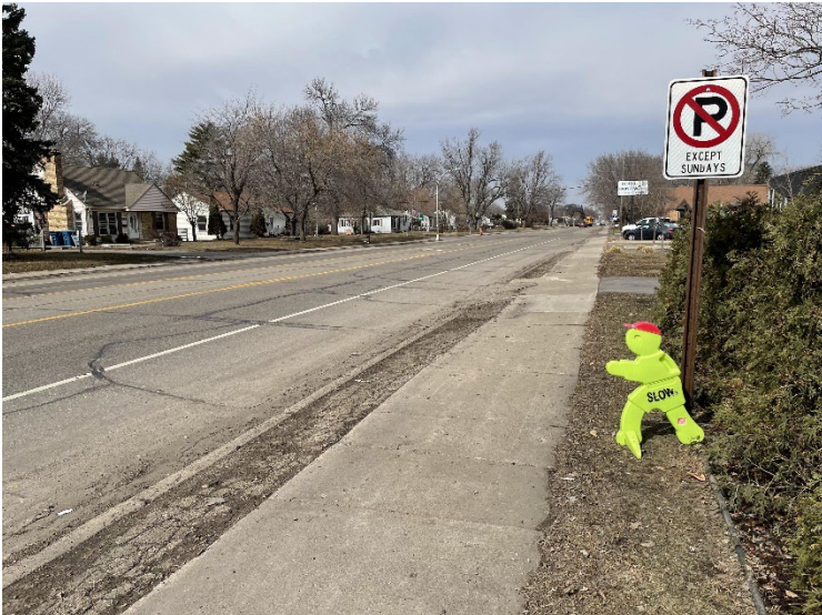
Wide curb-to-curb distances and high vehicle speeds make unsignalized pedestrian crossing difficult.
