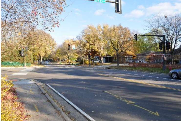
Figure 5 – Cedar Lake Road at Texas Avenue. No separation between travel lanes and pedestrians, no sidewalk on south side, crosswalk to no facility on south side, lack of APS facilities, no dedicated bikeway.
