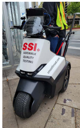
Figure A-4: Example of SEGWAY used to collect data
