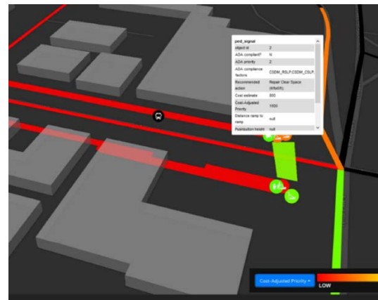
Figure A-7: GIS output showing processed LIDAR data depicting compliant and non-compliant sections of sidewalks and crossings
