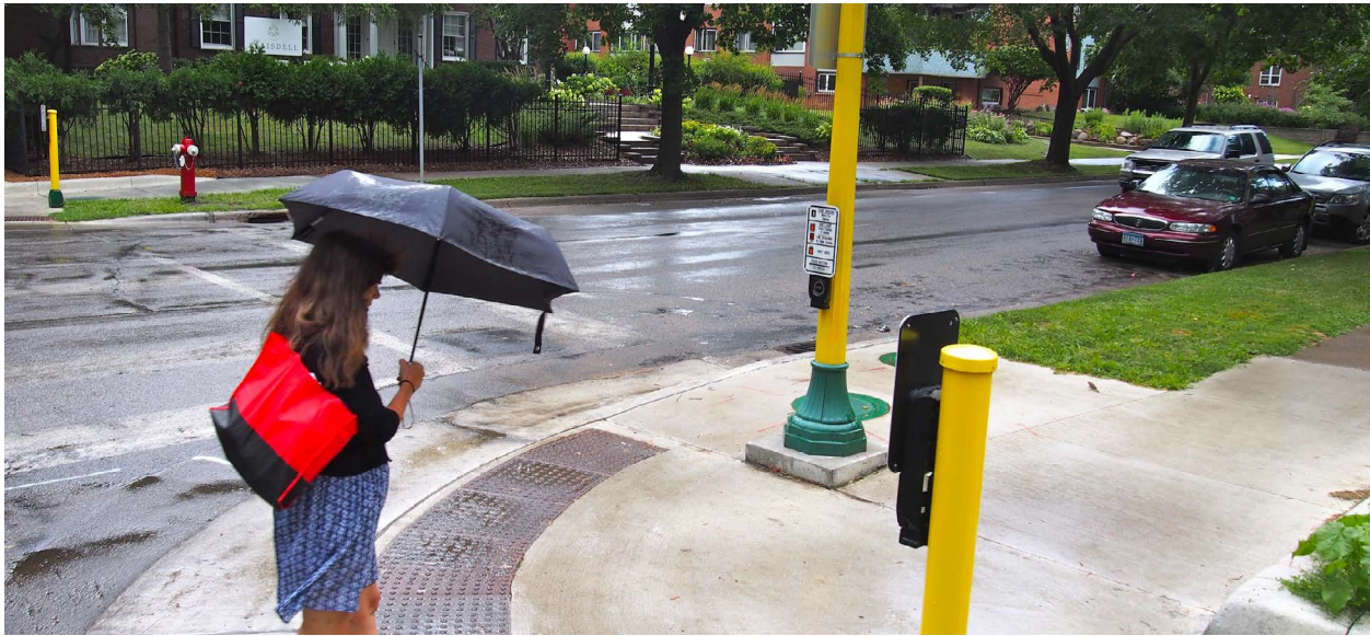
Figure E-1: Signalized intersection with Accessible Pedestrian Signal (APS) and pedestrian pushbuttons
