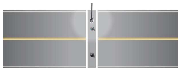
Midblock crossing with a single light
