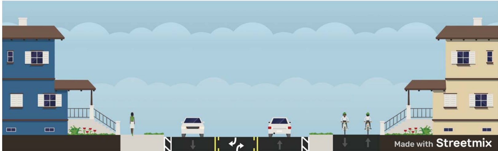
Figure 1 | Potential typical section along CSAH 5 (Minnetonka Blvd) from Xylon Ave to Virginia Ave
