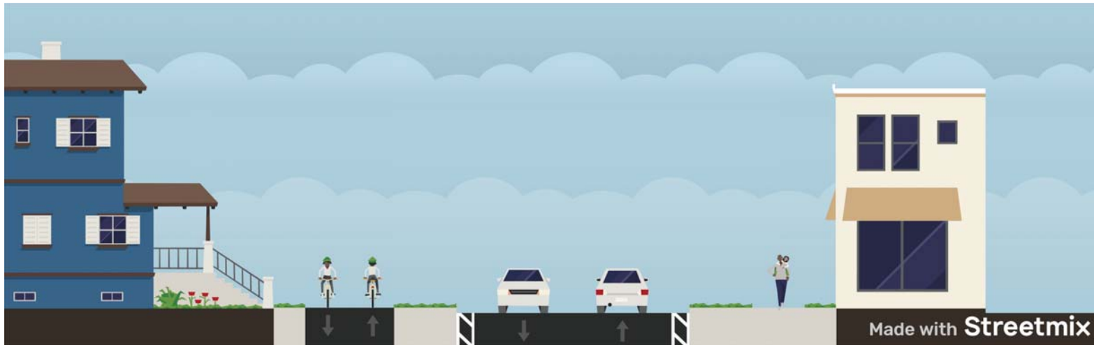
Figure 1 | Potential typical section along CSAH 153 (Lowry Avenue NE) from 50' East of Johnson Street NE to Stinson Parkway
