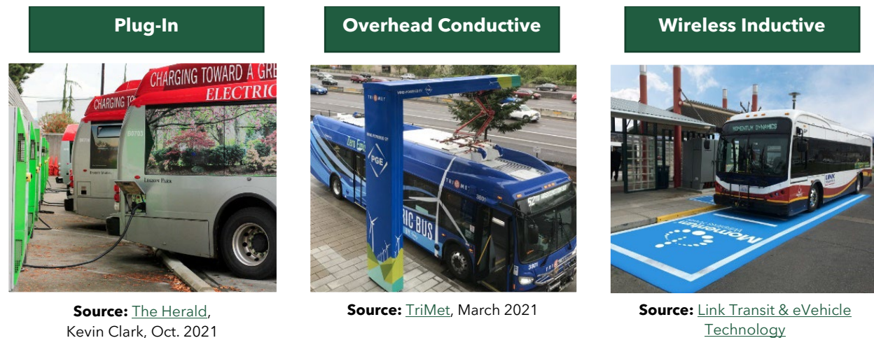
Figure 5: BEB Charging Infrastructure
