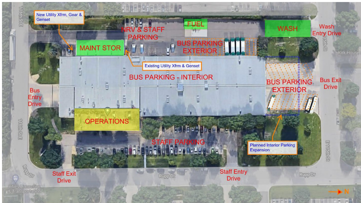
Figure 13: Burnsville Bus Garage Context Site Plan
